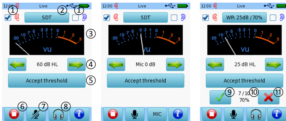
Figure 21: Live Speech user interface (left: SDT user interface with microphone turned off; middle: SDT user interface with microphone turned on and microphone level adjustment; right: WR user interface after accepting the determined threshold)
