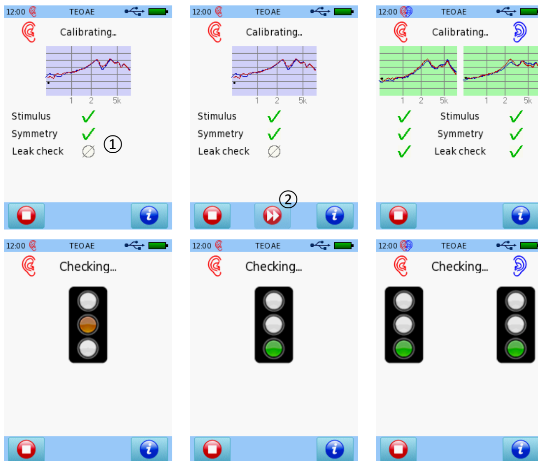
Figure 30: TEOAE ear probe calibration (top left: expert mode monaural; top middle: expert mode monaural with skip option; top right: expert mode binaural; bottom left/middle: simple mode monaural; bottom right: simple mode binaural)
