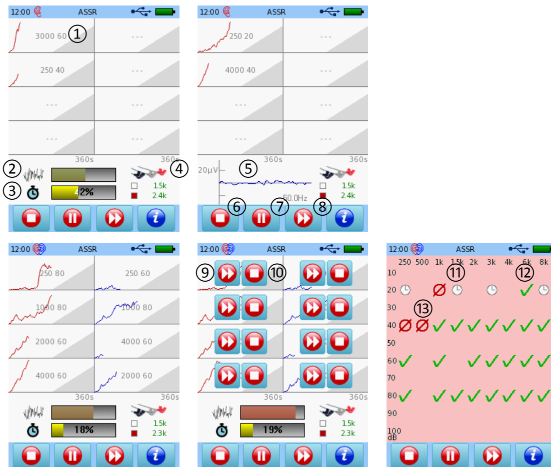
Figure 60: ASSR measurement (top: monaural 40 Hz ASSR measurement; top left: standard measurement screen; top right: measurement screen with EEG noise graph; bottom: binaural 80 Hz ASSR measurement; bottom left: standard measurement screen; bottom middle: skip/stop selection; bottom right: measurement status and result matrix)
